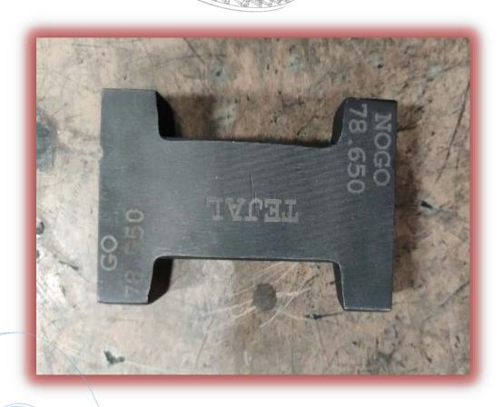
H-TYPE PLUG GAUGE IS USED TO CHECK THE PILOT BORE 100%
